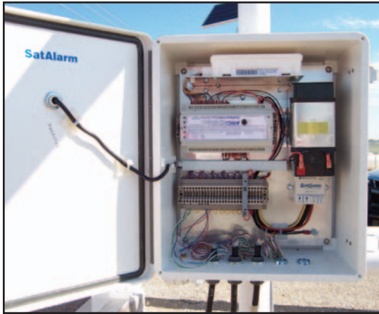
■ (Left) The Satellite Monitoring Unit (SMU) illustrated above includes a SatAlarm Interface Device (SID), satellite modem, terminal blocks and a backup lithium battery. (Right) This pole-mounted unit is equipped with American Millennium Corporation Inc.'s (AMCi's) integrated solar panel power supply.
